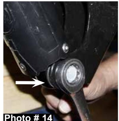
8. **G250 Kits:** Install the OEM rear coil spring isolators & OEM rear coil springs. **Note:** Be sure when installing the OEM rear coil spring isolators that the tab of each OEM rear upper coil spring isolator aligns with the hole of each new Skyjacker rear coil spring spacer.
