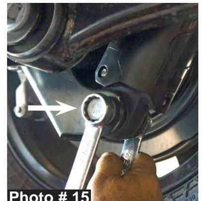
6. While checking for appropriate slack in ABS lines, brake lines, differential vent hose, & etc. Lower the rear differential & remove the OEM rear coil springs.
