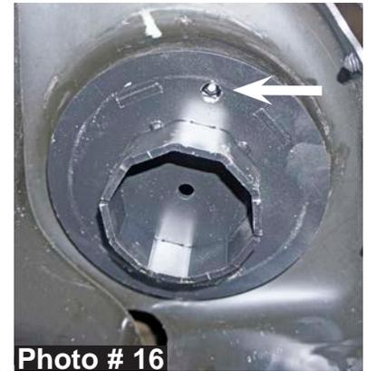
8. **Spacer Kits G250PELT & G250RPELT:** Install the OEM rear coil spring isolators & OEM rear coil springs. **Note:** Be sure when installing the OEM rear coil spring isolators that the tab of each OEM rear upper coil spring isolator aligns with the hole of each new Skyjacker rear coil spring spacer.
