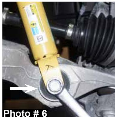
10. Remove the OEM upper A-arms using a 18mm socket / wrench.
