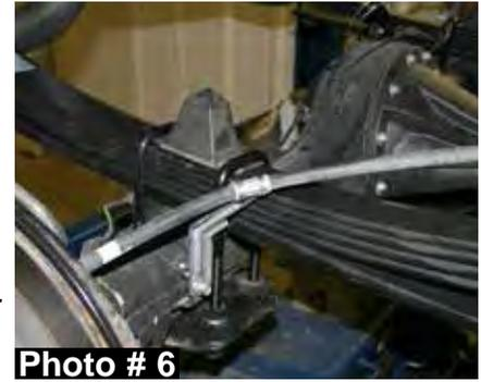
7. Install the new Skyjacker u-bolts using the supplied 9/16" fine thread nuts.
