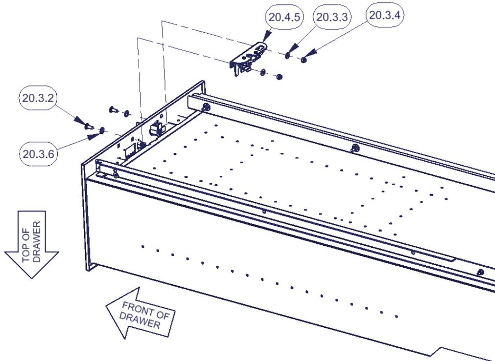
5. Install the #20.4.7 Combo Lock Drawer Handle to the front of the drawer and install with the (4) #20.3.2 carriage bolts, (4) #20.3.3 washers, and (4) #20.3.4 nuts (removed in Step 1). (Figure 5) **\*\*NOTE THE ORIENTATION OF THE HANDLE FITS OVER THE COMBO LOCK AND ORIGINAL PUSHBUTTON LOCK IN ONLY ONE WAY.**
