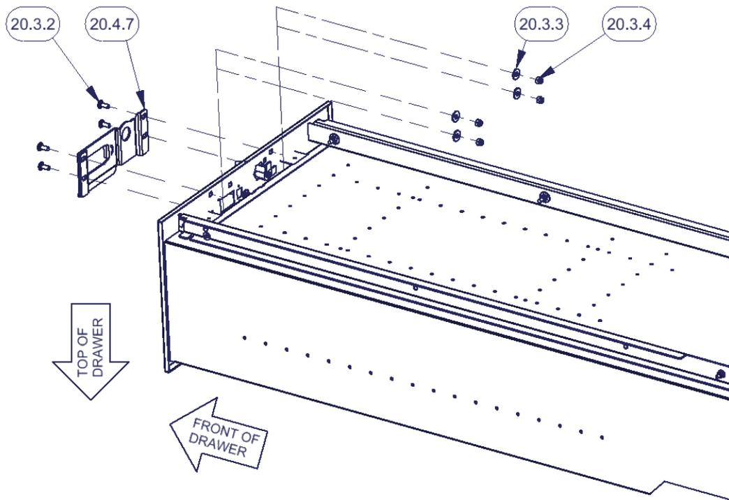
6. It is most convenient to set the combination lock code at this time. Refer to the document titled “**089 Operating instructions**” for instructions on setting combination code. **The combination pushbutton lock is typically shipped from the factory with either no code entered yet or “12345” and will need to be reset by the customer.**
