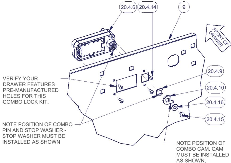
4. Install the #20.4.5 Combo Latch Assembly onto the drawer front panel by fitting it over the pushbutton and combo locks. \*\*This is performed on the inside face of the drawer. Fasten the assembly to the drawer front with the (2) #20.3.2 carriage bolts, (2) #20.3.6 rubber washer, (2) #20.3.3 washers, and (2) #20.3.4 nuts (removed in Step 2). (Figure 4)
