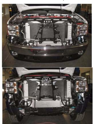
5. Remove four bolts from lower frame horn brackets.
