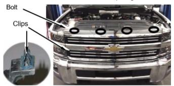
disconnect lower grille clips from core support to remove grille.
