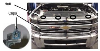
2. Install cover on core support with seven push pins.
