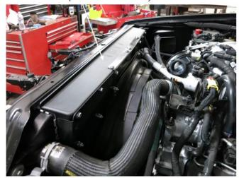
2. Reinstall fan/clutch, fan cage and secondary fan shroud as one assembly carefully back into vehicle.
