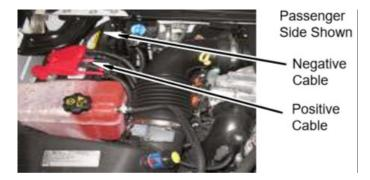
2. Install *kit* **extension bracket** (L-bent) using OEM nut onto battery terminal fuse junction and *kit* **hardware** (5/16") at positive cable end as shown below:
