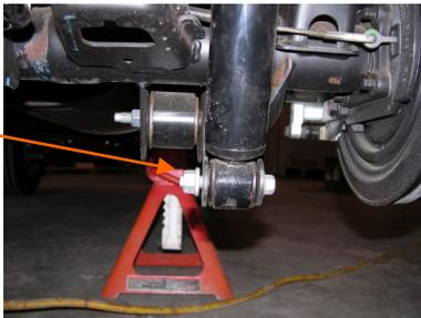
38. Disconnect the lower sway bar end link nut with a 16mm wrench.
