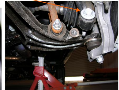
19. Remove the lower bolt at the lower control arm securing the clevis bracket with a 24mm socket.
