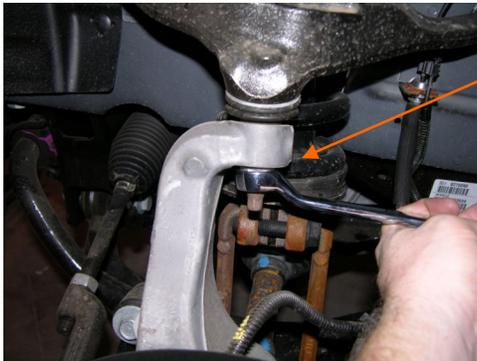
21. Pull downward on the knuckle to allow access to the strut.
