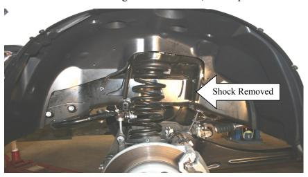
8. Disconnect sway bar end link at the axle. **Tools:** 21mm ratcheting box end wrench, 10mm open end wrench.
