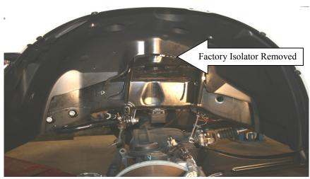
12. Remove the factory upper spring isolator. **Tip:** The Daystar leveling spacer's stud will locate using the same hole as the barb on the factory isolator.
