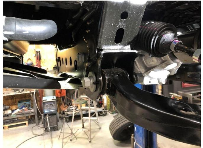
18. Torque the 2 lower strut nuts to factory specification, and torque the 3 upper strut nuts to 30 ft-lbs
