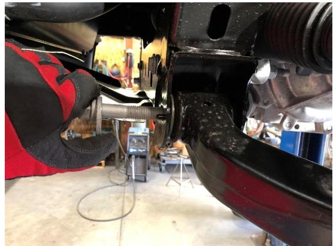
7. Lower the lower control arm to separate the strut from the lower control arm
