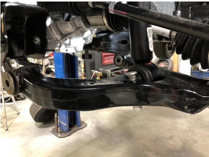
17. Raise the lower control arm and install the 2 factory lower control arm bolts at the frame
