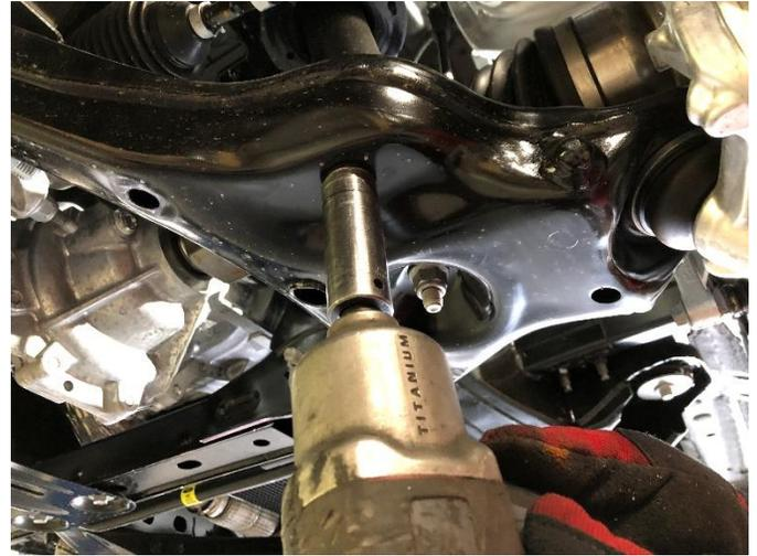
6. Remove the 2 factory lower control arm bolts at the frame
