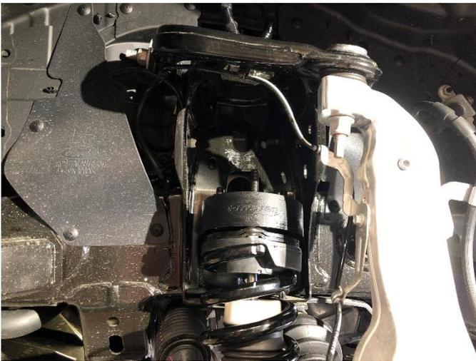
15. Align the 3 upper strut stud extension threads to the holes on the vehicle and fasten utilizing the provided kit lock nuts and washers
