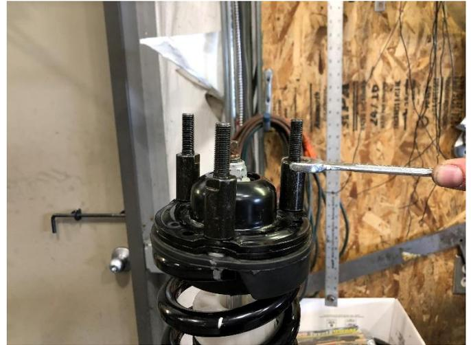
13. Install Daystar Strut Spacer to top of factory strut
