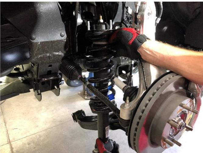
11. Remove the guide pin from the top of the strut assembly
