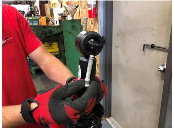
9. Remove the factory strut assembly from vehicle
