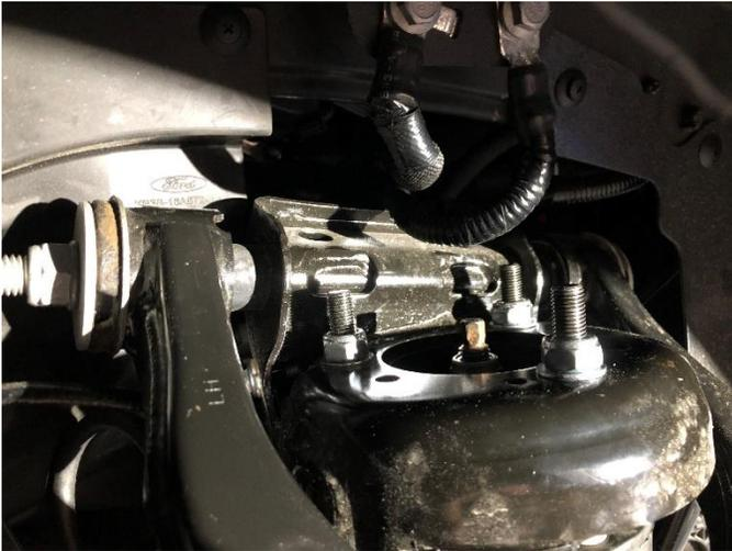
16. Install the 2 factory lower strut studs and nuts
