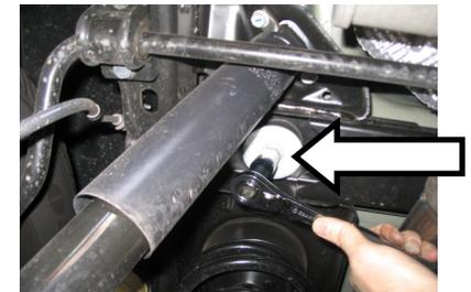
18. With the vehicle on the ground cycle the steering wheel side to side and inspect suspension components, brake lines and tires to ensure there are not any clearance issues. Jounce the suspension to assure front suspension operates freely, brake lines retain proper slack at full extension and that they remain clear of springs or other obstructions.
