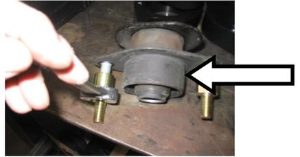
8. With the extenders tight install the body mount spacer over the stock mount.
