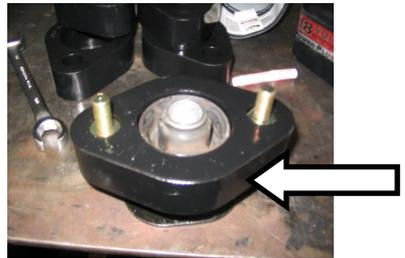
9. With the spacer mount installed. Install the mount into the fame support.
