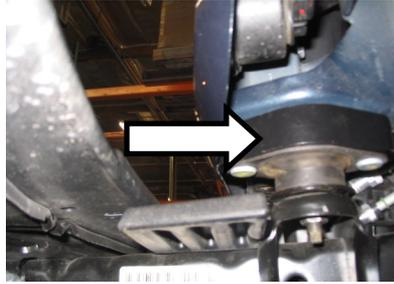
12. With all the body mount spacers installed remove the floor jack. use a 16mm socket and tighten all the 2 nuts per mount down to 40 ft lbs. Using a 18mm socket tighten down the 1 bolt per mount down to 80ft lbs.
