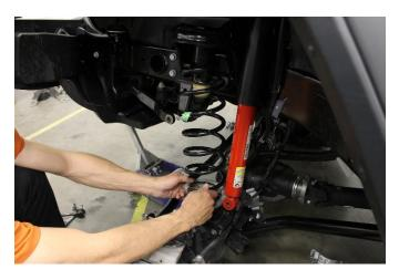
8. Install your new Daystar coil spring Spacer on top between the spring and the factory isolator.
