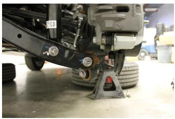
43. Torque the upper strut nuts to 30 ft-lbs
