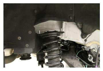
38. Install provided kit short Stud Extenders onto factory strut studs
