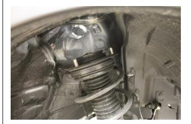
12. Install provided kit long Stud Extenders onto factory strut studs
