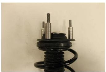
13. Install Daystar Front Strut Spacer to top of factory strut
