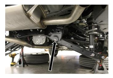
37. Remove both the factory lower rearward control arm bolt at the knuckle and the factory lower strut bolt, then lower the control arm and remove the factory strut assembly from the vehicle
