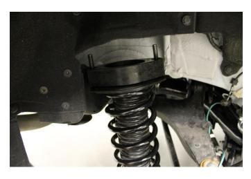
41. Align the 2 upper strut stud extension threads to the holes on the vehicle and fasten utilizing the provided kit lock nuts and washers
