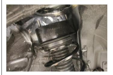
15. Align the 3 upper strut stud extension threads to the holes on the vehicle and fasten utilizing the provided kit lock nuts and washers
