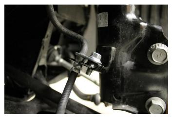
18. Install provided kit sway bar end link bracket onto strut, utilizing provided kit hardware
