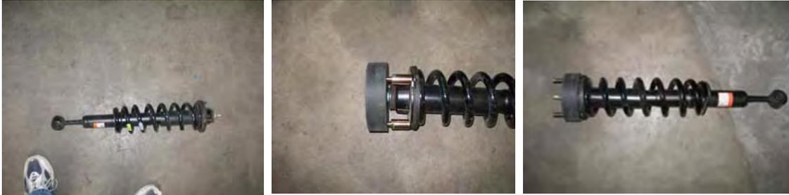
15. Reinstall the strut into the vehicle and tighten the upper strut nuts. You will have to push up on the upper a-arm to get the strut back in.
