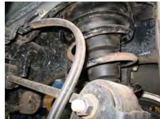
5. Jack up the rear suspension so the coil spring seats into the spring seat. Reconnect the lower shock and sway bar end , track bar and tires.
