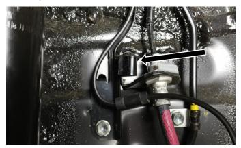
8. Remove / unclip factory brake line / ABS bracket / wiring harness from strut
