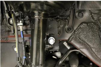
21. Install factory sway bar end link onto provided kit bracket
