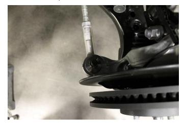
18. Install / clip factory brake line / ABS bracket / wiring harness onto strut
