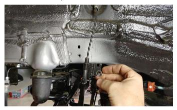
32. On the driver side, remove the factory fuel filler hose cover held in by 2 factory nuts and 1 factory plastic rivet
