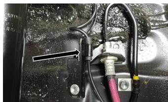
20. Install provided kit sway bar end link bracket onto strut, utilizing provided kit hardware
