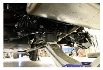
34. Remove rear subframe 2 factory front bolts and loosen 2 factory rear nuts
