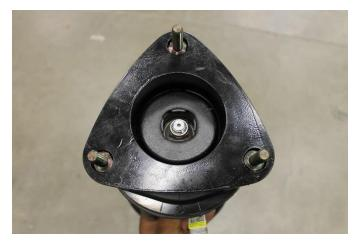
15. Install strut assembly onto vehicle, align the 3 upper strut stud extension threads to the holes on the vehicle and fasten utilizing the provided kit lock nuts and washers
