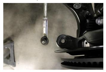
10. Remove the 2 factory lower strut bolts
