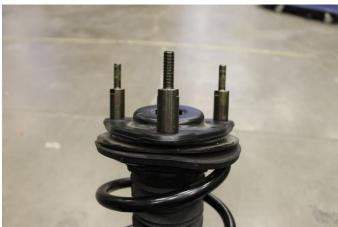
14. Install Daystar Front Strut Spacer to top of factory strut
