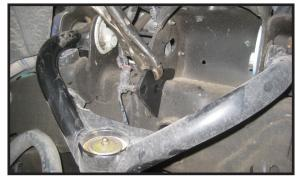
4. Using a 1/2" Drill bit, and the exising hole in the limiting strap bracket as a guide, carefully drill through the shock tower. Special Note: Due to tight quarters, this hole will most likely be drilled on a slight angle, and that is fine.
