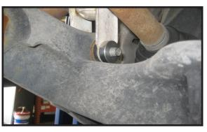
shock bolt, then install the nut.
