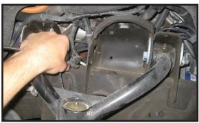
Locate the 13085-03 limiting strap brackets and insert them to the inside of the shock tower so that it follows the contour of the frame rail.
