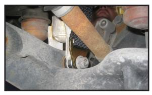
8. Using the 1/2 x 1 1/4" bolts and hardware, now attach the top of the limiting strap to the newly installed bracket.
