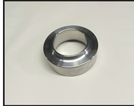
34105-04 / Qty. 2 Strut pre load spacer
