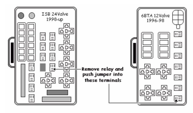
If the Engine Service Light comes on after operation, try reinstalling the relay then clear the fault code from ECM.
