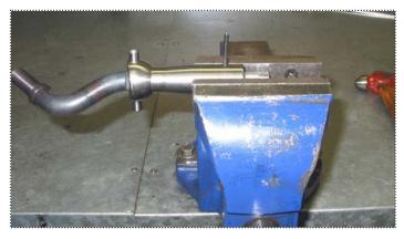
**NOTE:** The shifter rail pin has rubber Orings and lubricant used during assembly so it will be air-lock sealed in the shift arm assembly.
