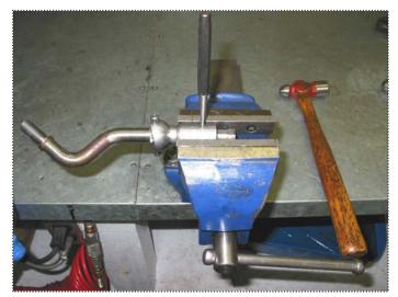
To change the shifter rail pin from the OEM shifter to the BD Short Shifter you will need to remove the shifter rail pin from the shift arm.
