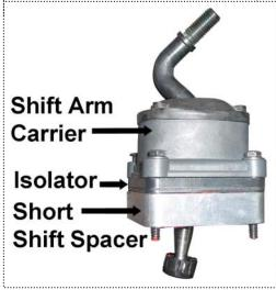
Install the shift arm carrier assembly onto the rubber isolator and install the four metal bushings in place. Insert and tighten the bolts with a 3/16" Allen socket to 7 - 9 ft lbs using a torque wrench.
