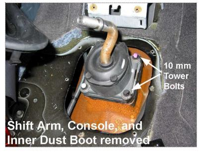
Remove the shift tower from the transmission.
