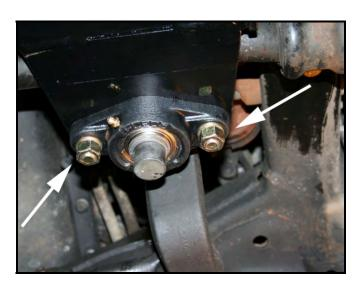
Remove the set screws and apply Loctite.
