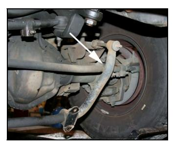
The 1-5/16" socket will be required to remove the steering box sector shaft bolt with lock washer. Retain the lock washer for re-installation with new nut.
