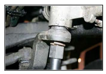
Slide the support bar into place, where the mounting feet are positioned in between the sway bar mounting and the frame. When the sway bar is moved into place the large diameter hole on the bearing plate will be approximately centered on the sector shaft nut.
