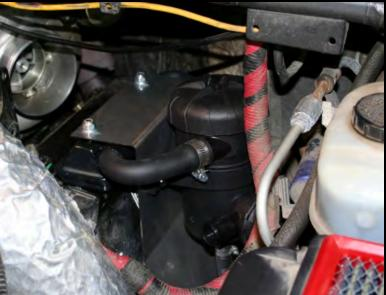
6. Install second hose (#**1302177**) onto snorkel. Secure this connection with spring clamp #24.
