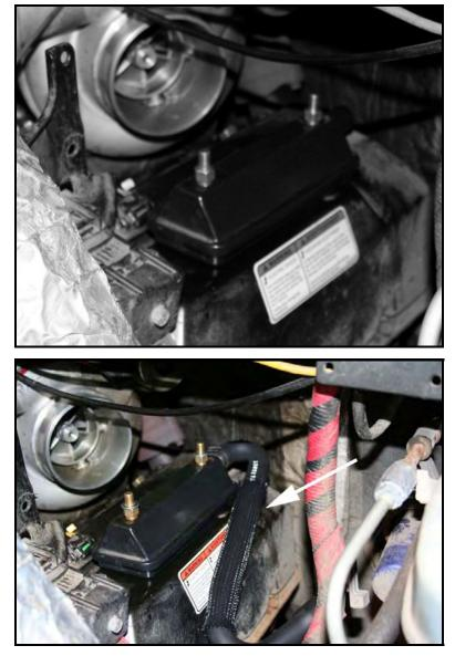
4. Install inlet hose (#**1302178**) onto breather vent. Use the #24 spring clamp (#**1302196**) to secure this connection.
