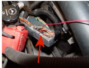
To activate the high idle, turn your switch into the ON position and switch the cruise to the ON position. This should result in an idle of 800RPM. Press the SET button on the cruise and the RPM should climb to 1200. Slide the switch to RESUME and the RPM should be at 1800.
