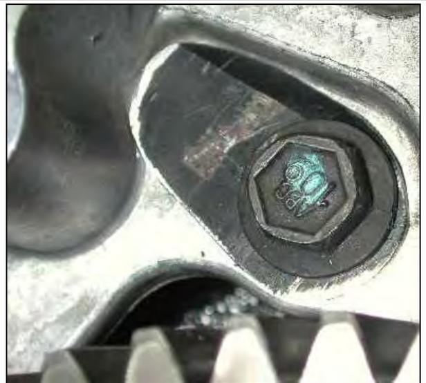
**With retainer and bolt installed**
