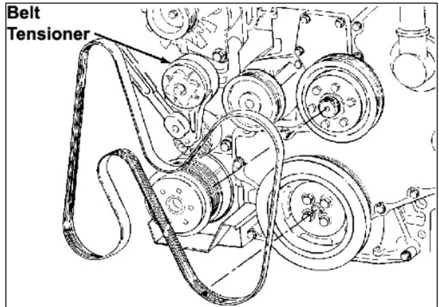
2. Remove the fan belt and the belt tensioner.
