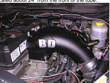
Move the intake around so that it is not touching anything and secure the intake with the supplied nuts. Note that the 12mm JIS nuts should be mounted to the smaller studs on the driver's side of the intake, while the 13mm Acorn nuts should be mounted to the longer studs. Be sure to place the washers underneath the Acorn nuts.
