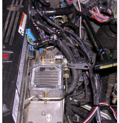
Place the new gasket (supplied) in place on top of the intake heater.
