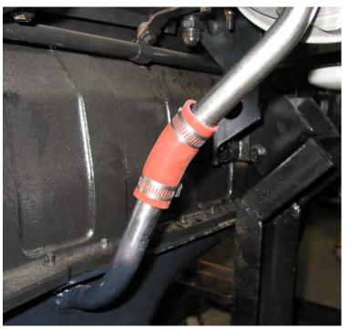
secondary turbo drain. This hose will attach to the factory drain adapter. Use the hose clamps to secure the connection. You will need to slide the oil drain adapter as far as possible away from the wastegate arm to prevent any contact. In some rare cases the wastegate arm may need to be bent.
