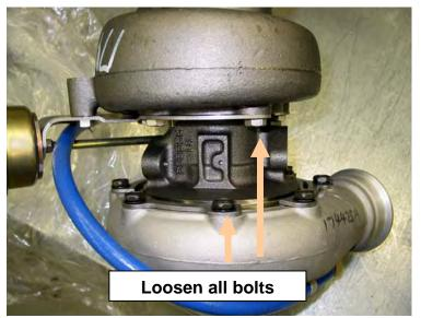
the turbo wheels. The clamps should only be loose enough to clock the housings.
