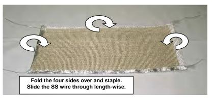
the silver side should be facing out, so that the tan wrap is fixed against the white side of the wrap. You will need to staple all four folds to secure them in place. Once secure, run the 40" stainless wire through the folds length-wise. You will need to do this on both sides.
