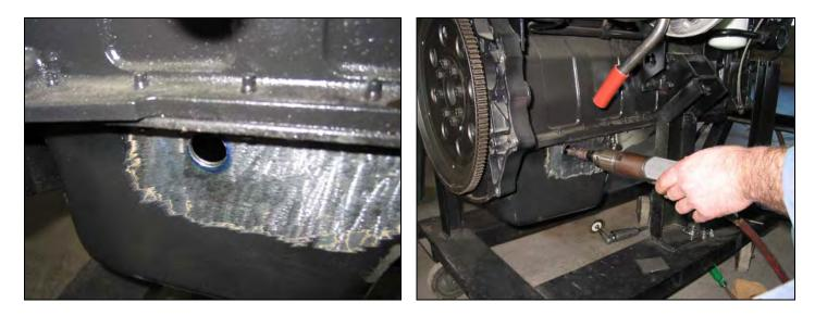
31. Center punch the pan 1 3/16" from top lip between the 3<sup>rd</sup> and 4<sup>th</sup> bolts
