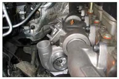
29. Using the supplied v-band clamp (clamp will be labeled 995L2-0406) secondary the tighten exhaust housing to the primary turbo-turbine adapter assembly.
