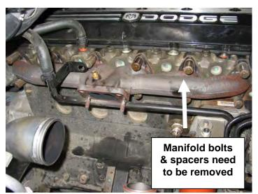
15. Reinstall the exhaust manifold in an **inverted manner** so the turbo flange faces upward. Use the provided manifold gaskets and the factory bolts, spacers and retainers and torque to 32 ft lbs with a 13mm socket.
