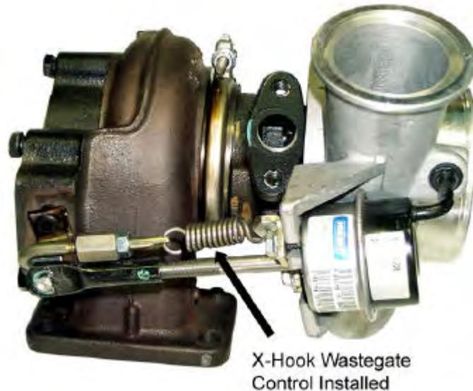
The BD X-Hook Wastegate Control bolts onto the turbo housing and controls the waste gate lever by increasing the pressure on the valve.
