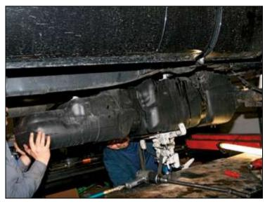
Rotate the locking clip that secures the basket to the fuel tank.
