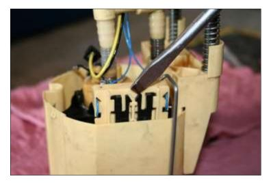
Release the two locking clips that secure the float with a flat head screwdriver.
