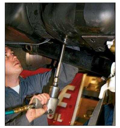
Raise fuel tank back up into vehicle and reconnect all connections. Secure the tank to the vehicle.
