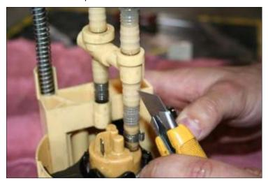
With a sharp knife, score the plastic tube to release the outer tube and expose the 3/8" barb.
