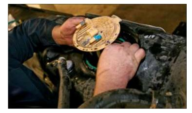
With the basket removed, use a hack saw blade and cut the three supports from the OE lift pump.
