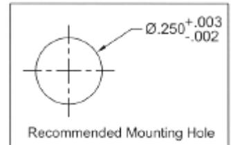
**IT IS CRITICAL THAT YOU CORRECTLY DRILL THE ¼" PERFECTLY 90° OR PERPENDICULAR TO THE DRILLING SURFACE.**
