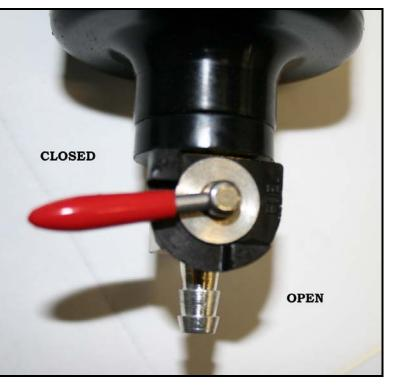
To drain the oil catch can, turn the lever to the open position.
