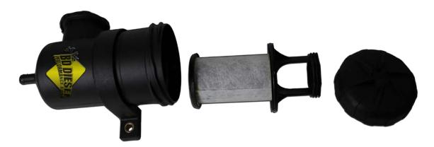
To change the filter unscrew the cap off of the canister, grasp the handle on the filter & pull it out of the canister. It should come out with a firm tug.
