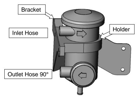
7. Install the Outlet Hose (bent hose ends 90°) to the bottom (Outlet) of the CCV Bottle with a #32 spring clamp.
