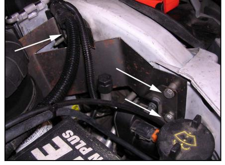
6. Install CCV canister into the bracket (#1302180) using the provided 5/16" hardware. You may have to undo the latch on the plastic canister holder & clock the canister to match what is shown in the illustration. Then install the canister & bracket assembly into the vehicle using the bolts for the radiator support.
