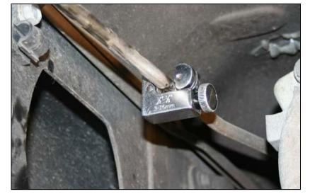
14. Route the fuel line that you connected from the front of the vehicle to the outlet of the pump. Use a hose clamp to secure this connection. Trim to fit, the remainder of the hose will be used for the inlet of the pump.
