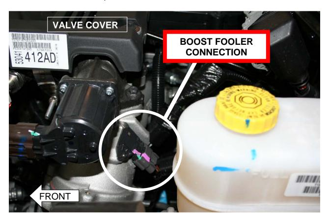
Unplug the factory boost connection from the engine. Plug the BD Boost Fooler inline with the factory plug, and then plug the remaining end of the BD Boost Fooler into the factory plug on the engine.
