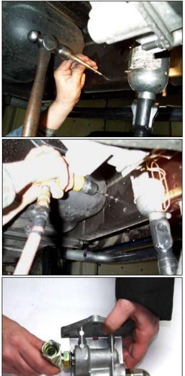
To allow for easier drilling, center-punch the two marked spots for the mounting bolts.
