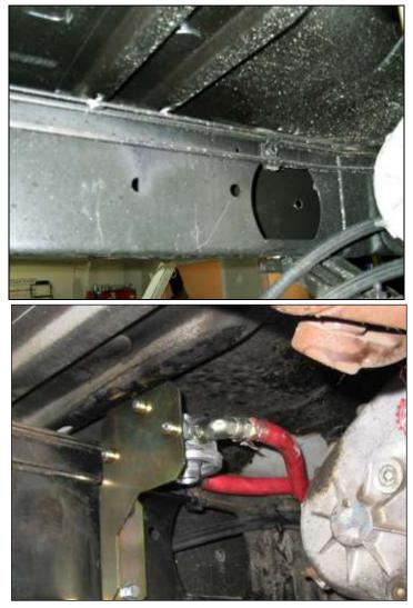
Locate and clean a spot to mount the filter housing along the left hand (driver side) frame rail.
