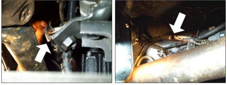
Using a small pipe cutter, cut the line approximately 6" from the bend. NOTE: You may want to use the drain pan to capture any spilled fluid.
