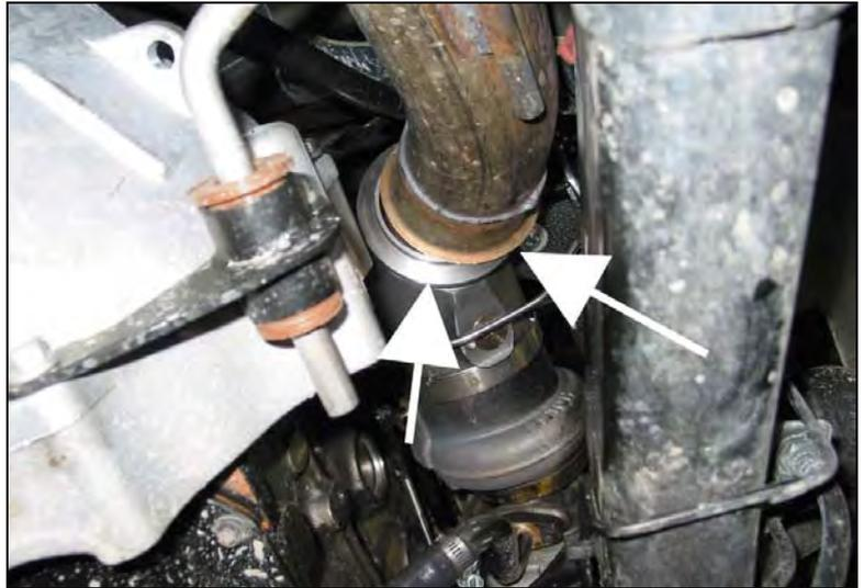
Remove the exhaust elbow.
