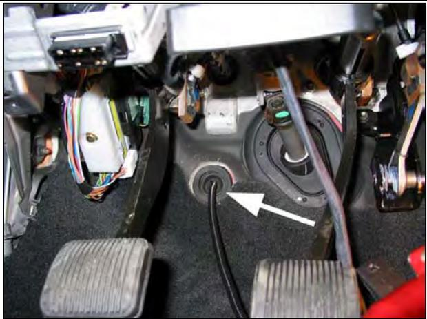
**ACCELERATOR PEDAL POSITION SENSOR (2004½-05)**
