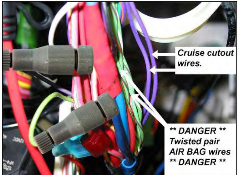
In this same wiring harness, locate the **violet w/ Brown tracer** wire and install another gray Posi-Tap. Insert the **green** wire from the DFIV module into this connector.
