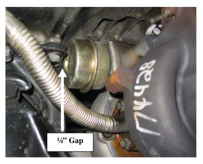
re-installing the intercooler tube, rotate the tube so that it is clear and free from the air box and the plastic inlet tube. Be careful that the compressor outlet elbow does not contact the shock tower.
