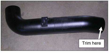
before re-installation into the 4"-5.5" silicone boot. Use the previous 4" gear clamp to secure the boot onto the inlet tune. Reconnect the filter and Air Mass sensor.
