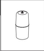
**1** Insert the top of the flattened air spring into the coil spring through the lowest opening with the air inlet at the top, as shown.
