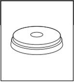
**1** Install the spacer on top of the air spring, as shown.
