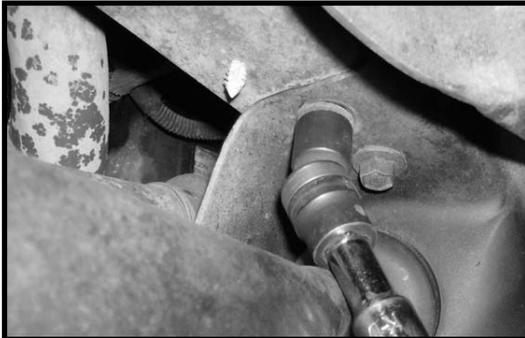
4. Working on the driver side, carefully drill out the frame and the stock radius arm bracket holes to 1/2". Repeat procedure on the passenger side.
