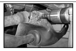
cation brackets. Also, locate (16) 1/2" x 1 1/2" bolts, (32) 7/16" USS flat washers and (16) 1/2" unitorque nuts from hardware and add some tread locker or loctite and torque to 65 ft lbs. Repeat procedure on the passenger side.
