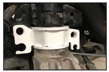
11. Locate (2) 9/16" x 1 1/2" bolts, (4) 1/2" SAE washers, and (2) 9/16" unitorque nuts from hardware bag 42103NB. Install the new hardware into the new strut spacers and torque to 125 ft lbs.
