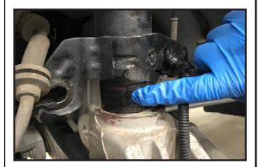
8. Locate the correct strut spacer halves according to the photo below. Special note: The install photos we have used here, are of the passenger side.
