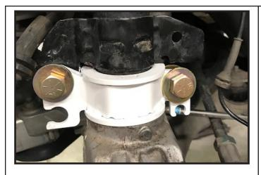
12. Install the OE brake line and ABS wire into the slots of the new strut spacer pieces.
