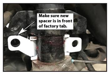
10. Install the outer spacer and ensure all holes align with the inner spacer and factory bracket. The upper and lower "C" shaped pieces should contract each other after wrapping around the body of the strut.
