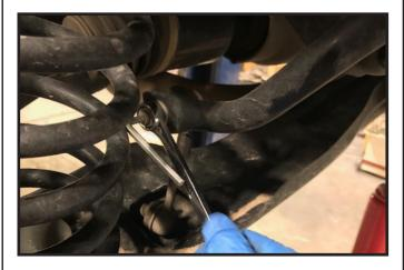
22. Place a jack under the lower control arm, raise the jack up until there is light pressure on the lower control arm but not raising the vehicle. Remove the lower contro arm bolt that attaches to the knuckle.
