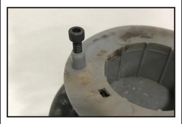
25. Install the new rear coil spacer by placing it over the locating dowel on the lower coil spring isolator so that the #10 bolt peeks through.
