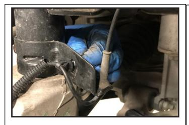
6. Using a dead blow hammer, carefully hit the top of the knuckle until it has slipped down approximately 1 5/8".
