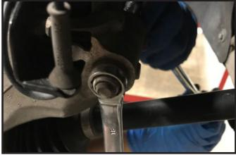
5. Remove the ABS wire from the strut mount and carefully move the ABS wire out to the side.
