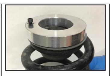
26. Locate the small locating hole in the lower control arm, and install the new coil spring spacer/OE isolator/coil spring assembly so that the #10 bolt falls into the locating hole on the lower control arm.
