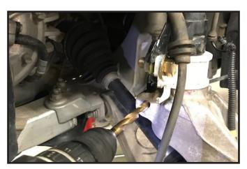
15. Locate and install the new 7/16" x 3" bolt, (2) 3/8" washers, and 7/16" unitorque nut. Torque to 55 ftl lbs.
