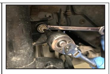
4. Using an E14 socket and an 18mm wrench, remove the knuckle pinch bolt that clamps the knuckle to the strut. An 11mm 12 point socket can also be used if you are careful.
