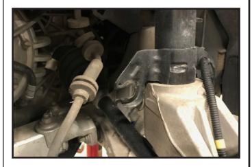
3. Remove the sway bar endlink from the strut mount. Use a 5mm Allen wrench to hold the stud from turning.
