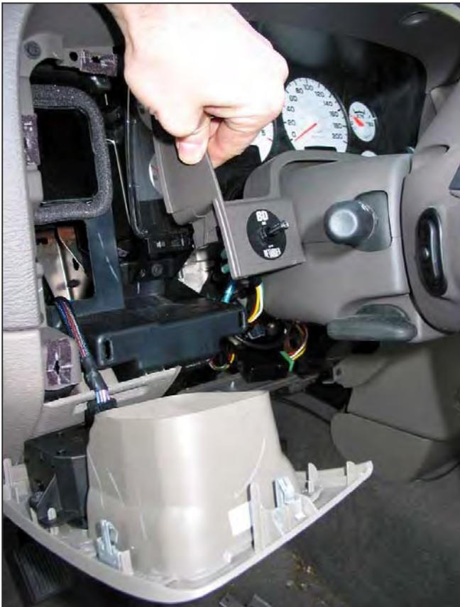
Install switch into drilled hole and secure with lock ring then reinstall dash trim panels by reversing the removal procedure.
