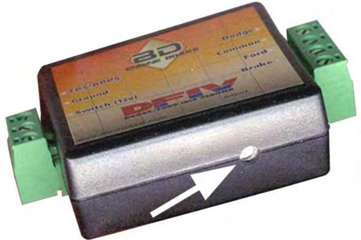
**CAUTION:** THE ADJUSTING SCREW IS A MICRO-SWITCH THAT IS VERY DELICATE, SO TURN USING SMALL ADJUSTMENTS.
