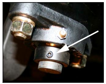
Check that the zerk grease fitting is tight. Use a standard grease gun to apply grease to the bearing.
