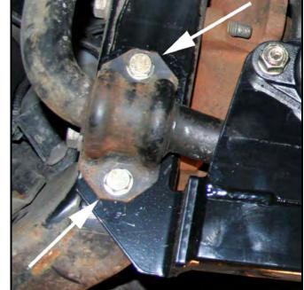
Remove the set screws and apply lock tight.
