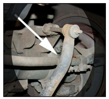
Allow the sway bar to swing down and rest on the steering linkage.
