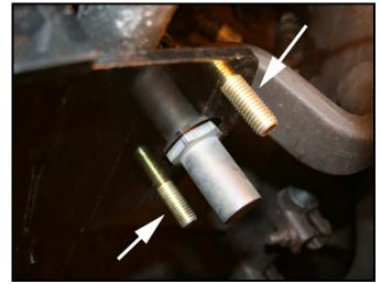
Install two bolts through the small holes in bearing mounting area, so that the threads are hanging through the bracket.
