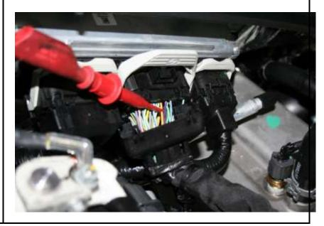
17. Being that the RPM signal is critical you will need to solder the connection.
