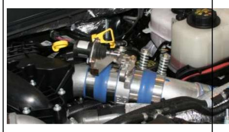
11. Lay out supplied harness over top of the driver's side of the engine.
