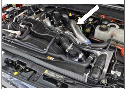
3. Once the pipe is removed from the truck, you can make your first cut at 4 1/2" from the factory pipe benders grip start on the C.A.C. side.
