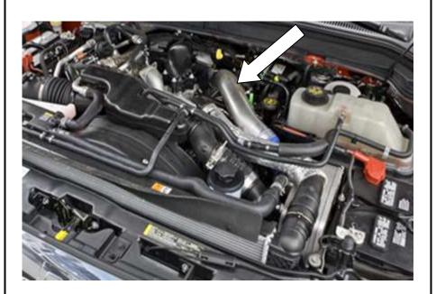
3. Once the pipe is removed from the truck, you can make your first cut at 4 1/2" from the factory pipe benders grip start on the C.A.C. side.
