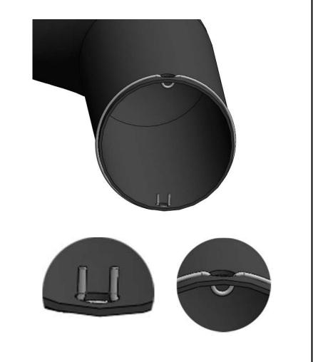
Once the bead rings are installed, connect the pipes to the valve assembly ensuring the arrow on the valve points towards the pipe that connects to the turbo.
