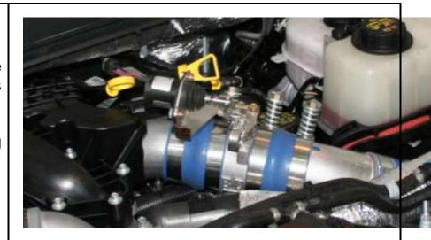
12. Lay out supplied harness over top of the driver's side of the engine.
