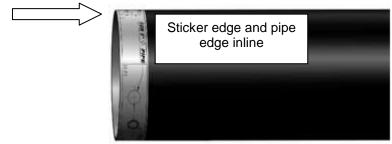
6. With the sticker in place use a center punch and then use a Ø1/8" drill bit and drill a hole in the center of the holes marked "For 3Ø".
