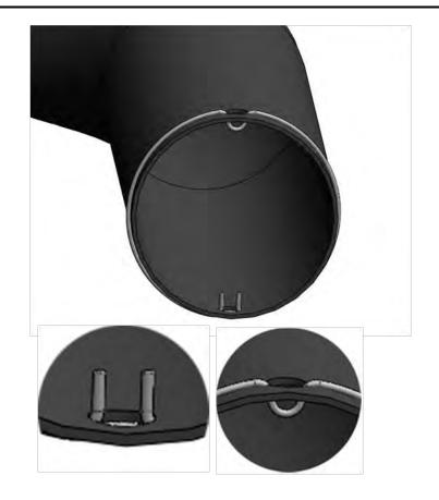
10. With the holes and bead rings installed in both pipes you can now install the silicone boots and then the positive air shutoff valve.
