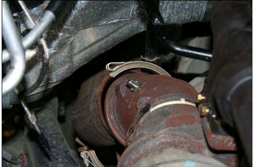
Disconnect the compressor outlet boot.
