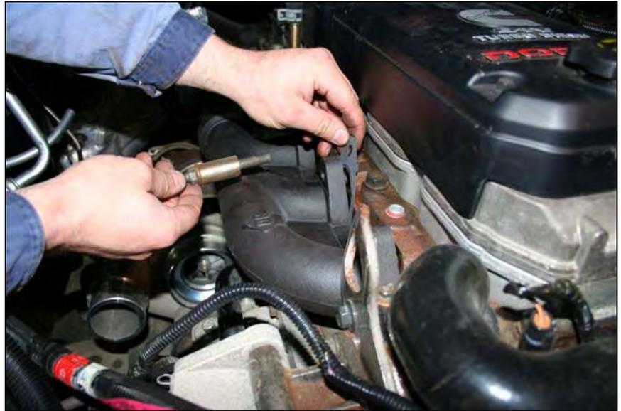
When installing the lower bolt to cylinder #5, discard the factory bolt and spacer. Place the coolant pipe bracket against the manifold and install the **M10 SS socket head bolt (1405981)** and the **M10 Washer (1405982)** to secure the bracket and the manifold to the head.
