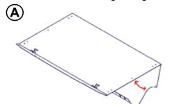
Rotate Hinge to open top and front panel
