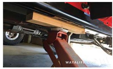
Note: Use a towel, rag or 2x4 between jack and rocker to avoid scratching the powdercoat.
