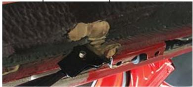
Cut off the 6 rocker trim mounts from the pinch seam.
