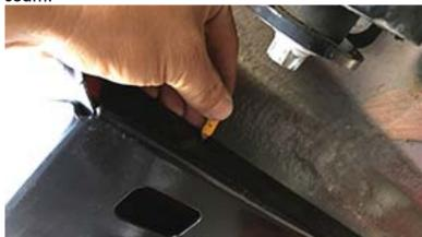
5. Using a 5mm allen wrench, remove the bolt next to the "NO STEP" warning label that secures the plastic rocker trim to body of your Renegade.
