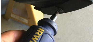
4. Located on the bottom of Renegade's plastic rocker trim, you will find 6 plastic fasteners securing it to brackets extending from the pinch seam. Use a flathead screw driver to lower the fastener locking pins remove the fasteners from the plastic rocker trim.
