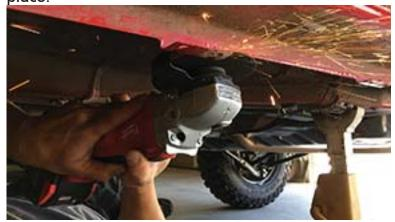
Note: When the glue is removed and the front and rear tabs that held the plastic panel are trimmed off, the rocker will fit snuggly against the bottom of floor behind the pinchweld, the bottom of the rocker and the door jamb; there will be no doubt that it is in
