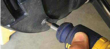
Remove the screw securing the rear end of the plastic rocker trim to the inner fender liner and body.
