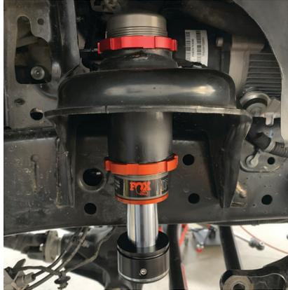
Fig. 5: Install the lock rings.
