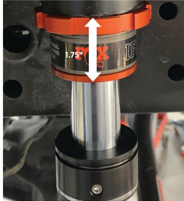
Fig. 6: The bearing cap must protrude 1.75\".
