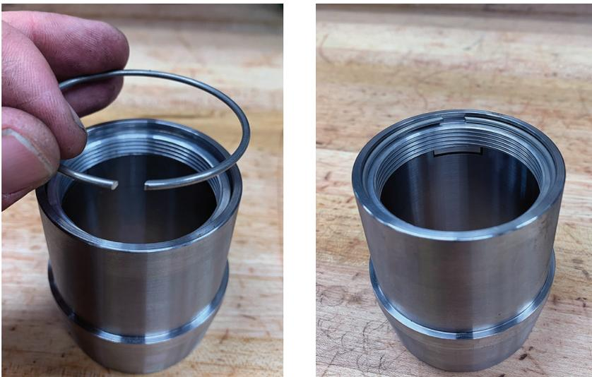
Figure 9: Installing the wire snap ring
