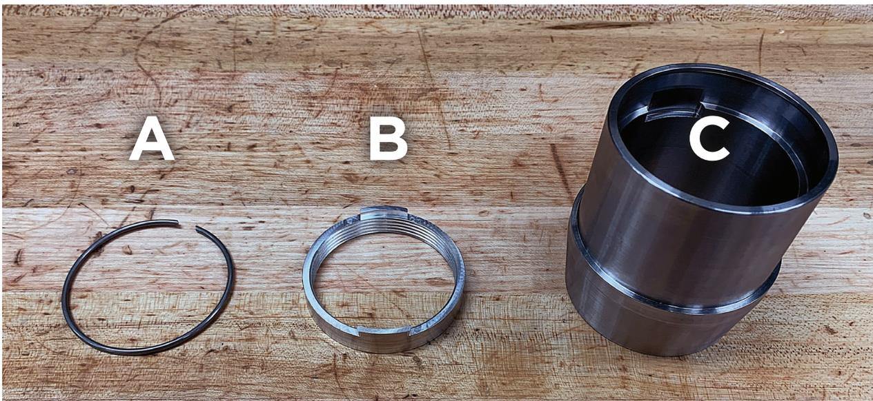
Figure 7: Bump Stop Holder Parts
