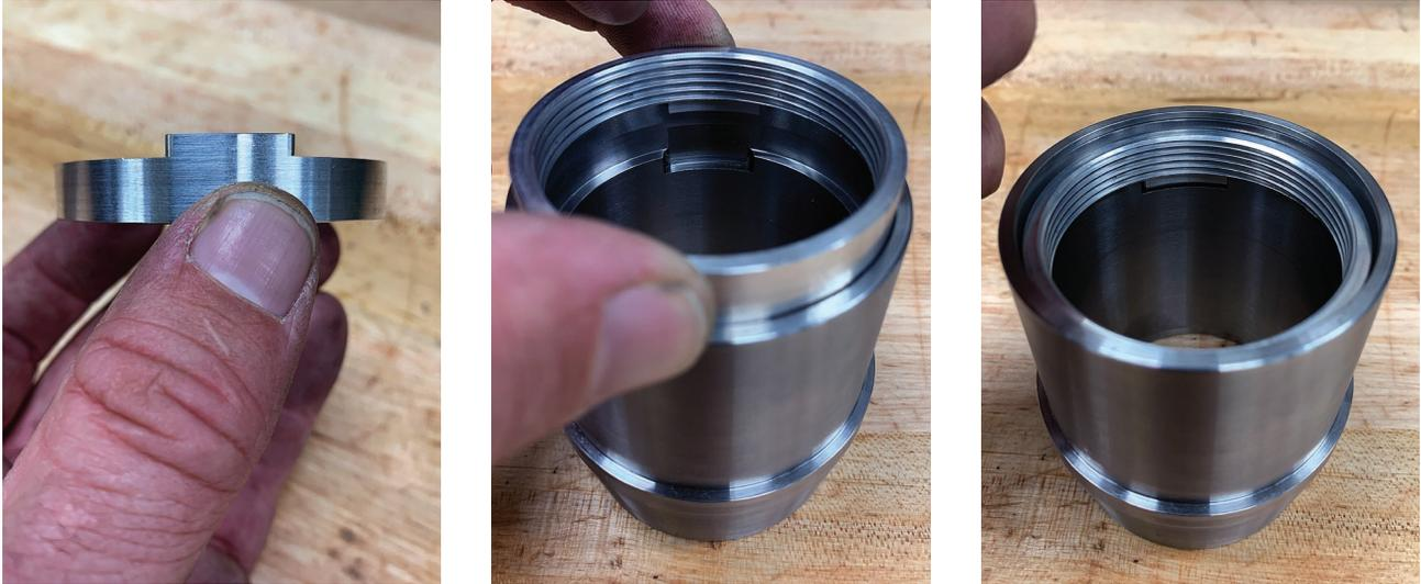
Figure 8: Installing the threaded aluminum ring into the steel weld in bump stop holders
