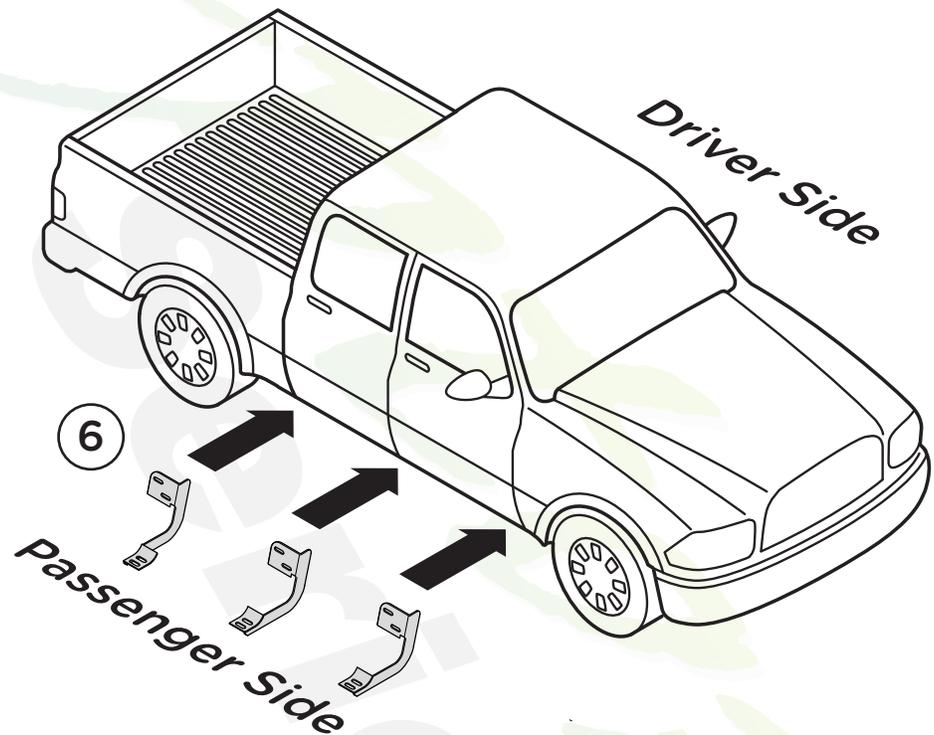
**7.** Line up each bracket to the 12 Bolt + M10 Nut Plate located in the rocker panel.
