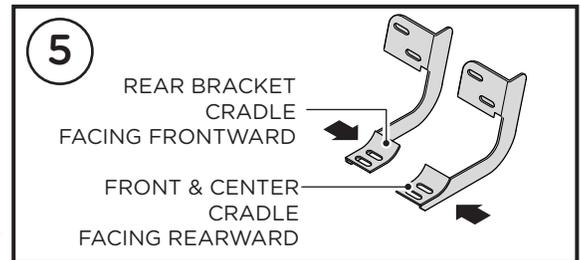
**6.** Begin installation on passenger side. Position Front Bracket, Center Bracket and Rear Bracket as shown along passenger side.
