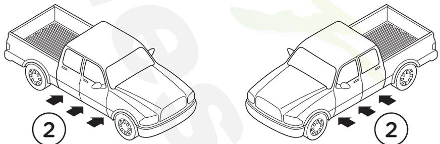
**3.** Remove the **Tape** covering the factory oblong hole in the rocker panel located above the two (2) hex holes.
