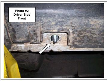
**Step-2** Attach the driver side front auxiliary bracket to the rocker panel using the 5/16" t-bolt, (1) 5/16" flat washer, (1) 5/16" lock washer and (1) 5/16" hex nut, (**Photo #3**). Leave the hex nut loose for final adjustment.
