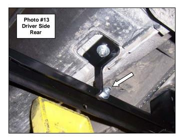
**Step-11** Set the driver side, side bar on top of the brackets and align the side bar with the vehicle. Position the clamp brackets inside the opening of the side bar and align the clamp bracket threads with the slot holes in the brackets. Attach the side bar to each of the brackets using the clamp bracket, (2) 5/16" x 1" square head bolts, (2) 5/16" lock washers and (2) 5/16" flat washers, (**Photo #14**). Leave the square head bolts loose for final adjustment.
